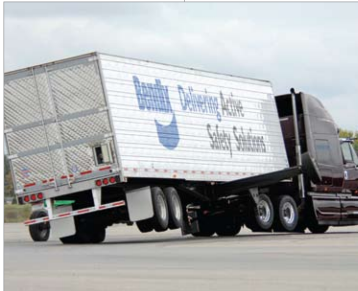
Bendix ESP deploys both roll and directional stability to help mitigate rollovers, as well as the loss-of-control events that often lead to rollover.
