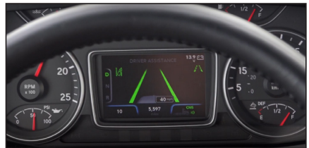
Figure 2 - Green lane lines show the system is tracking the lanes and may intervene if needed.
