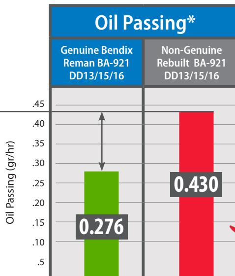
\*Higher levels of oil passing may cause downstream contamination and potential component failure.
