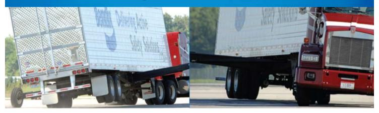
Bendix TABS-6 Advanced is a single-channel option for trailer roll stability. The system evaluates conditions, such as those pictured here, that may lead to a rollover, and intervenes by automatically applying the trailer brakes.
