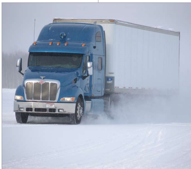
Only full-stability technology, such as Bendix ESP, is capable of intervening to mitigate potential jackknife and loss-of-control situations on both dry pavement and on slick, low-friction road surfaces such as those that are wet, icy, or snow-covered.
