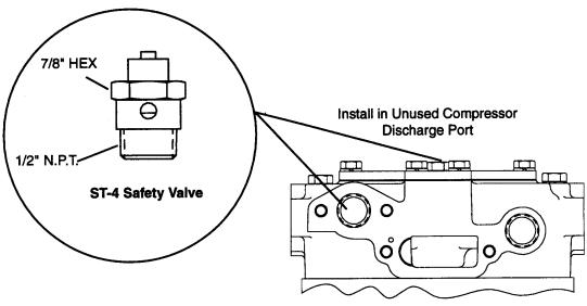
**Typical Compressor Cylinder Head**
