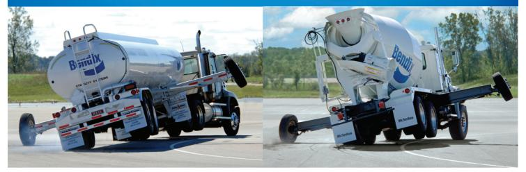
Bendix® ABS-6 Advanced with ESP® is a full electronic stability technology that mitigates under-steer, over-steer, and rollover situations like those pictured above.
