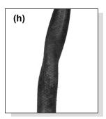
Partly collapsed inlet line shown.
