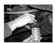
Drain <u>all</u> air tanks (reservoirs) into the Bendix<sup>®</sup> BASIC<sup>™</sup> test cup. (Bendix kit P/N 5013711).
