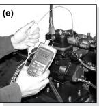
Testing the temperature at the discharge fitting.
