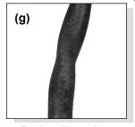
Partly collapsed inlet line shown.
