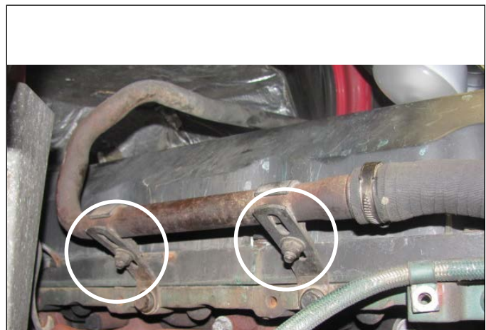
Figure 16 – Air Intake Pipe Adjustments
