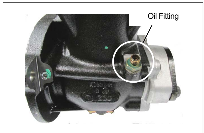
Figure 6 – Oil Fitting Installation
