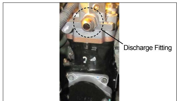
Figure 7 – Discharge Fitting Installation
