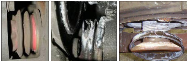
Typical Evidence of thermal overload Evidence of thermal overload
