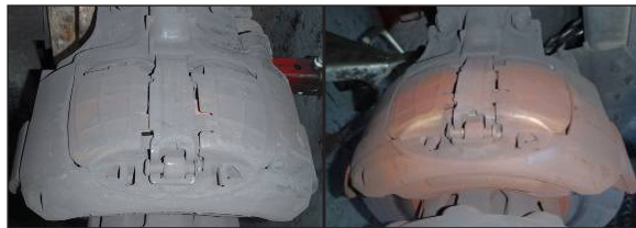
Normal Evidence of thermal overload
