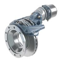
Before mounting the Spring Brake Actuator on the ADB Caliper, the front Mounting flange surface (in contact with the ADB Caliper) must be inspected and cleaned.
