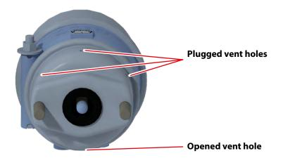
It is recommended by Knorr-Bremse to plug any other vent holes with plugs (included in the service kits) to decrease dust and water continual ingress inside of the NPP.
