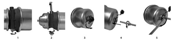
Set that the Hand brake valve lever in the "run" position (parking Air Disc Brake Calipers in "released" position). Air connection Port 12 is with Air pressure now.
