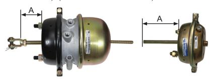
Push rod length 'A' is measured from the bottom of the actuator to the end of the push rod. This dimension is taken with the spring brakes released or caged.
