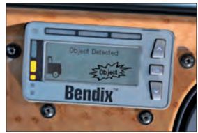
Example of Stationary Object Alert Display
