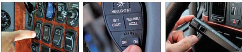
Examples of cruise control switches
