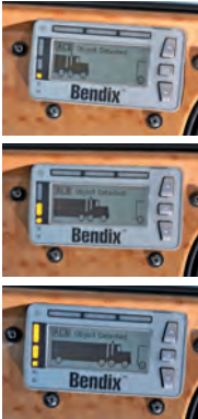
Above: Driver Interface Unit (DIU) – Showing Examples of Following Distance Alerts – with progressively faster audible alerts.
