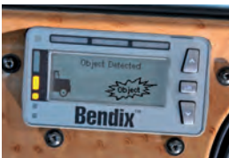
DIU: Showing Stationary Object Alert – a continuous tone will also sound.
