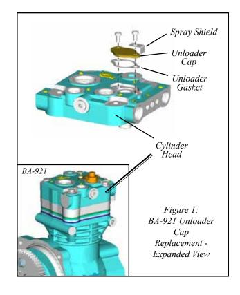
Where a **spray shield** is already installed, the unloader cap upgrade has already been made, and **no action is needed**. Only the BA-921 compressors listed below are part of this service campaign.
