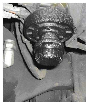
Air dryer exhaust with oil present
