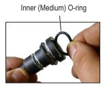
4. Lubricate the entire ESS piston assembly as shown below. Pay special attention to lubricating the three (3) installed o-rings.
