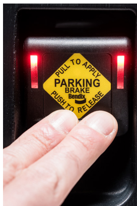
PUSH the DECU switch to release the parking brakes.
