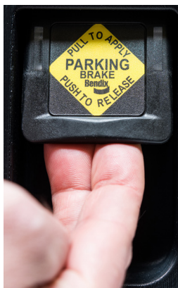
PULL the DECU switch to set the parking brakes.
