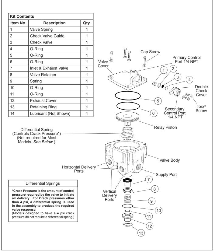
Figure 1 – Bendix® R-12DC® Relay Valve Exploded View
