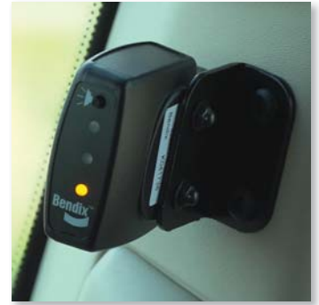
Yellow = System is active; no detectable objects in the blind spot; safe to make lane change (driver should double-check the mirrors and activate vehicle's turn signal first)
