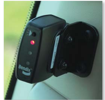
Red = A vehicle is likely within, or nearing, the truck's blind spot; exercise extra caution; it is not yet safe to change lanes
