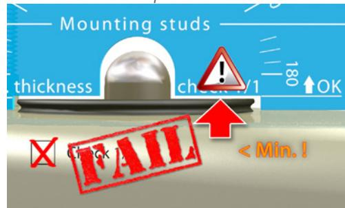
The height of the seal should not drop below 3 mm. If the seal height is lower than the line marked "min. thickness check 1/1", the check has failed.
