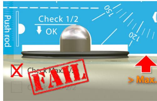
If the gauge does not lie flat on the actuator due to interference with the push rod the check has failed.
