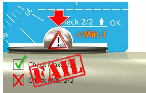
If the push rod height is lower than the "OK" line, the check has failed.
