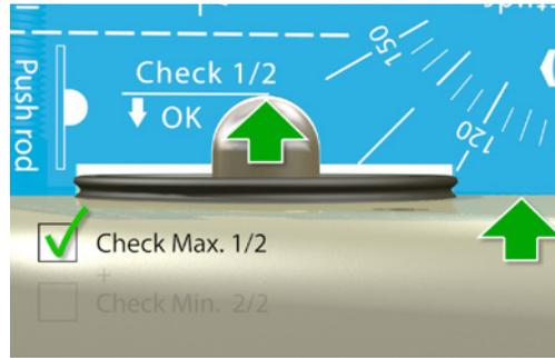
If the gauge lies flat on the actuator and there is no interference with the push rod, the check has passed and you should move on to test for minimum permitted height.
