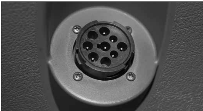
FIGURE 7 - TYPICAL VEHICLE DIAGNOSTIC CONNECTOR LOCATION (J1939)
