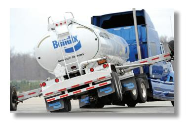
Bendix® TABS-6™ Advanced roll stability system provides trailers with core antilock braking, along with Trailer Roll Stability Program (TRSP®), in one efficient package that's simple to install and simple to maintain.
