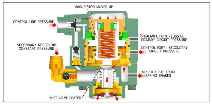
FIGURE 9 - SERVICE APPLICATION LOSS OF PRIMARY CIRCUIT
