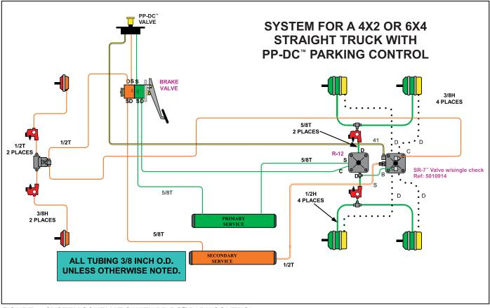
FIGURE 3 - SYSTEM SCHEMATIC WITH PP-DC<sup>™</sup> PARK CONTROL
