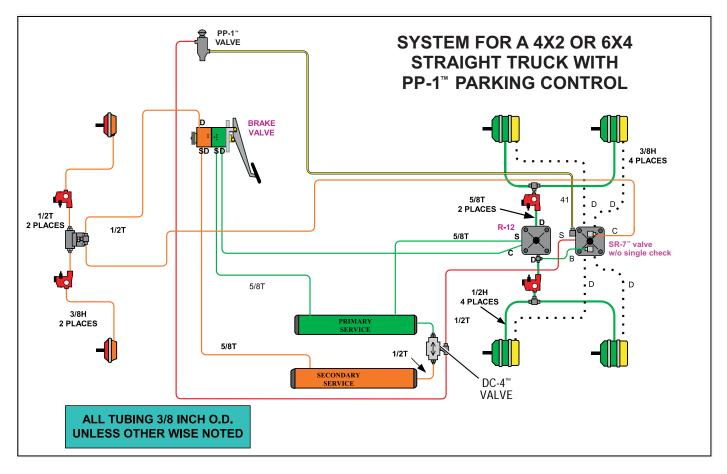
FIGURE 4 - SYSTEM SCHEMATIC WITH PP-1<sup>™</sup> PARK CONTROL AND DC-4<sup>™</sup> DOUBLE CHECK VALVE
