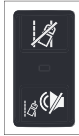
Figure 28 - LDW, HDW, and HDB Disable Switch
