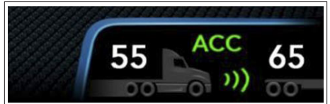
Figure 5a - ACB Actively Engaged and Maintaining Set Following Distance
