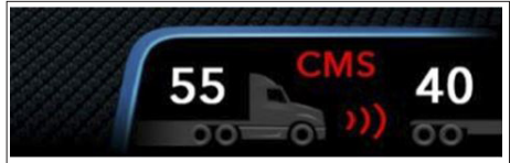
Figure 12b - AEB System Alert and Possible Autonomous Braking Applied
