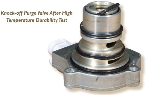
*The knock-off's* purge valve fell out of the dryer prior to completing the test.
