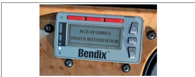
FIGURE 12 – ALARME DE FREINAGE EXCESSIF
