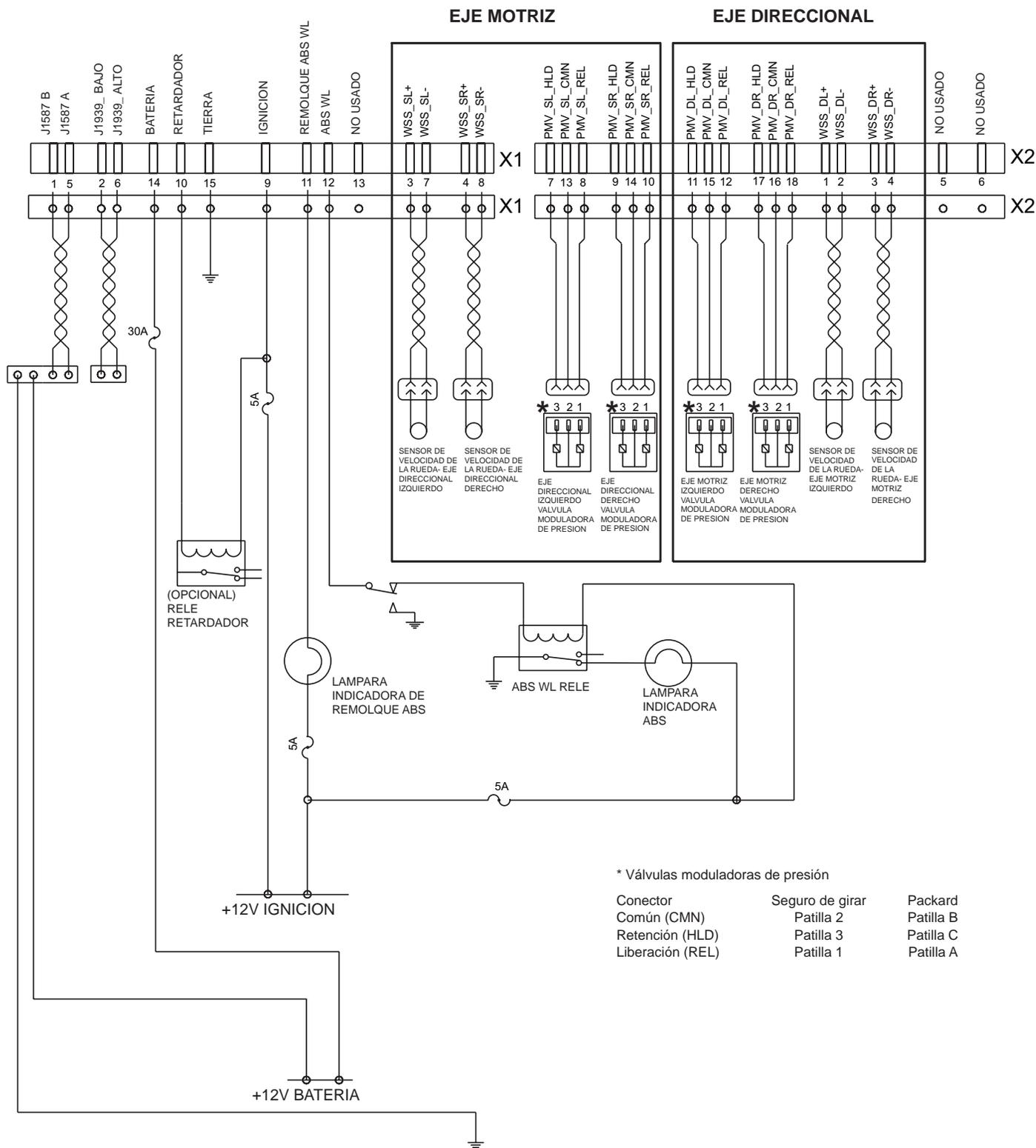
FIGURA 19 - ALAMBRADO ESQUEMATICO DE CHASIS ESTANDAR (4S/4M)
