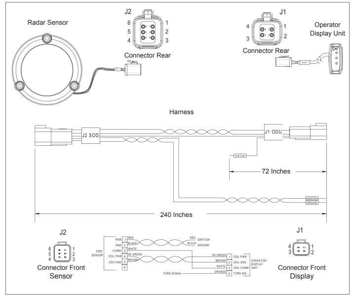
Figure 8 - Harness Electrical Diagram
