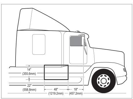
Figure 4 - Recommended Installation Location (Single Sensor Systems)
