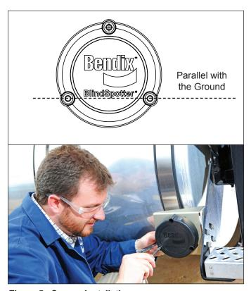
Figure 5 - Sensor Installation
