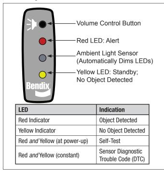
Figure 3 - Bendix BlindSpotter Driver Display Unit LED Indicators
