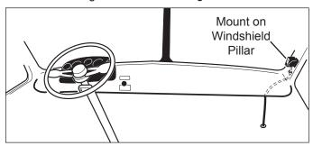
Figure 6 - ODU Installation
