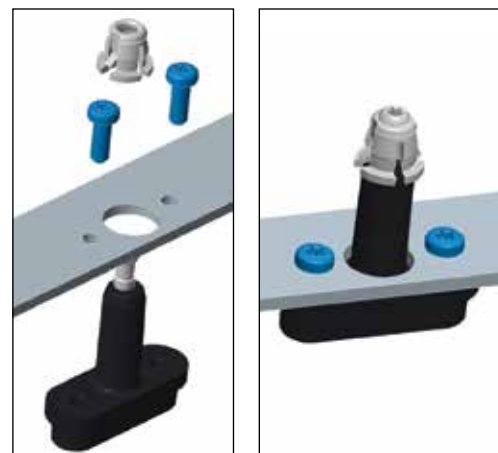
FIGURE 4 - RADAR SENSOR ADJUSTERS INSTALLATION
