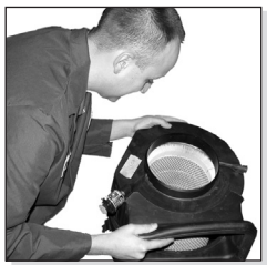
Inspect the engine air cleaner.
