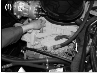
Inspecting the coolant hoses.
