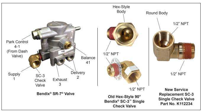
Bendix is aware that certain vehicle applications can cause the hex-style 90° elbow SC-3 check valve to wear prematurely and contaminate the SR-7 valve, causing a small reservoir leak through the SR-7 valve exhaust.
