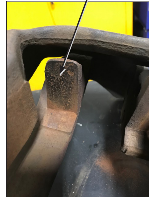
Abutment Surface Rust Removed
