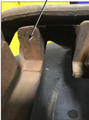
Abutment Surface Rust
