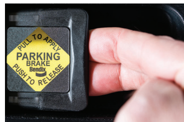
PULL to APPLY parking brakes
