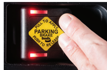
PUSH to RELEASE parking brakes
