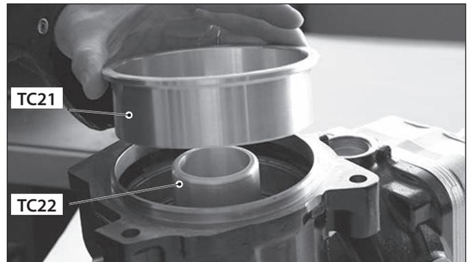
Disassemble the bearing by separating the inner ring with balls from the outer ring
