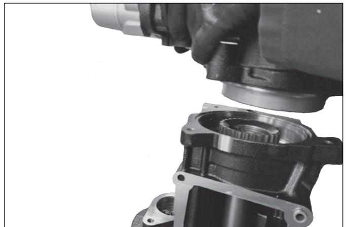
Align the two units with one another and screw together using the 3 screw fasteners (36) - torque **50 Nm**.
