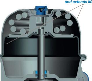
Electroless/nickel park side push rod reduces the risk of leakage
