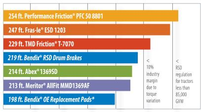
Source: Bendix testing. Stopping distances are simulated based on FMVSS-121 Hot Stop and Recovery. \* Result achieved with Bendix\* BX276™ OE replacement pads.
