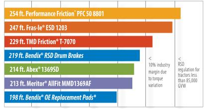
Source: Bendix testing. Stopping distances are simulated based on FMVSS-121 Hot Stop and Recovery. \* Result achieved with Bendix<sup>®</sup> BX276<sup>™</sup> OE replacement pad.
