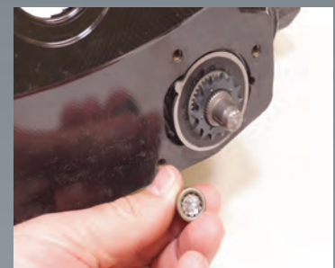
Failed adjuster / Requires caliper replacement
