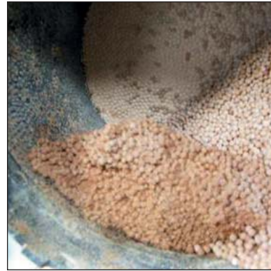
Competitive desiccant after testing. Beads are clumped, powdering into the air system.
