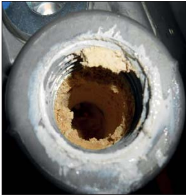
Partial blockage: the port is partially blocked and air is restricted due to desiccant failure. Mitigate blockage with the Bendix GC cartridge, a reliable solution at a great price.
