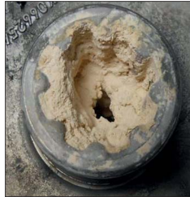
Full blockage: the port is full of clumped desiccant. Blockage can cause the air brake controls to fail. The system will likely have to be flushed and components replaced (thousands of dollars in repairs) plus downtime.
