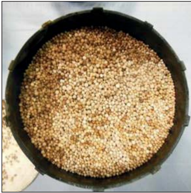
Bendix desiccant after testing. Beads are intact with no clumping or powdering.
