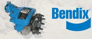
Bendix ADB22X Air Disc Brakes – Heavy Duty Stopping Powerand Durability with Passenger Car Feeland Control
