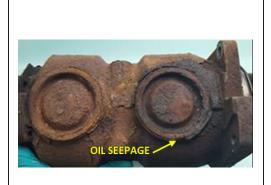
**Figure B:** Example of twin-cylinder compressor with bottom cup plug exhibiting corrosion and oil seepage.
