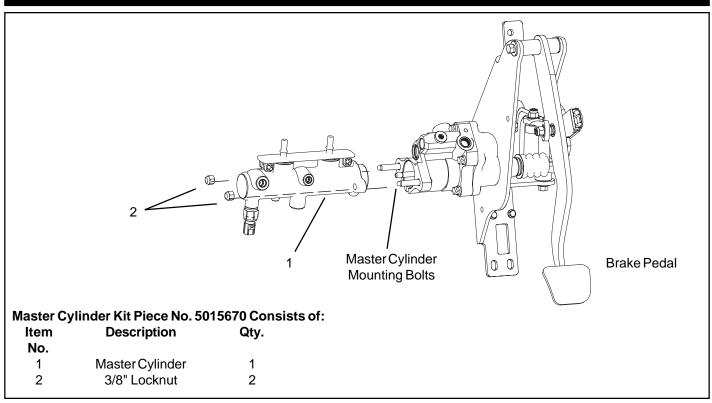
Figure 1 Blue Diamond Brake Control Module
