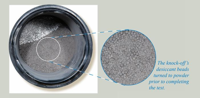
The inferior desiccant in this knock-off dryer – bought right off the shelf – delivered 35% less drying capacity and was easily fouled by oil, reducing dryer life by 50%. In addition, when desiccant beads turn to powder, contamination results - leading to downstream component malfunction or failure.
