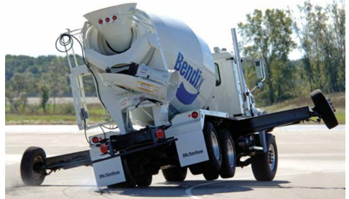
Does more than just rollover mitigation – Bendix ESP also addresses many of the "loss of control" situations that can lead to rollovers or other accidents.
