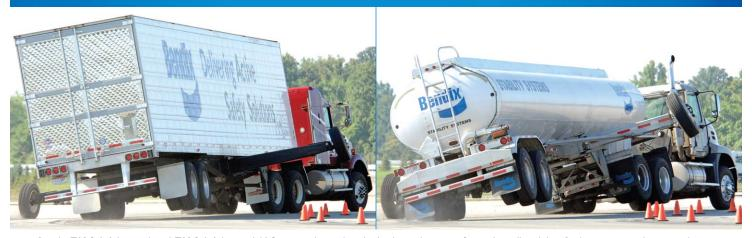
Bendix TABS-6 Advanced and TABS-6 Advanced MC are single- and multiple-channel options for trailer roll stability. Both systems evaluate conditions, like those pictured here, that may lead to a rollover, and intervene by automatically applying the trailer brakes.
