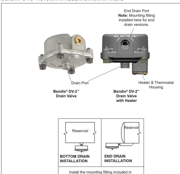
**NOTE**: When installing automatic drain valves equipped with a heater and thermostat, connect the #14 gauge heater wire to the 'on' position of the engine control or ignition switch. Use an 8 amp fuse for one valve, a 15 amp fuse for two valves, and a 20 amp fuse for three valves. All electrical connections must be waterproof.
