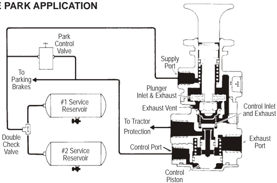
FIGURE 7 - PP-7™ TRAILER SUPPLY VALVE PARK APPLICATION
