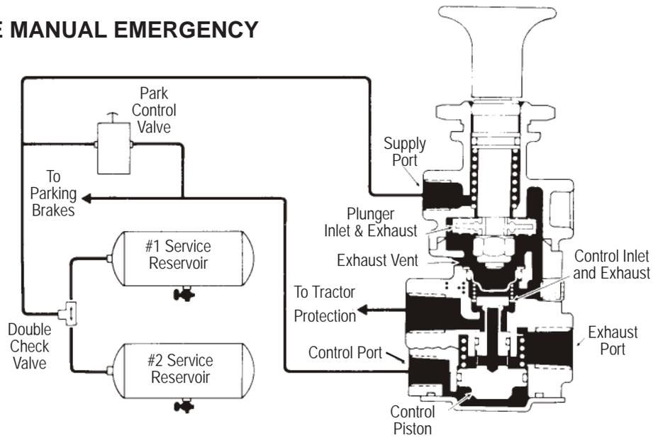
FIGURE 6 - PP-7™ TRAILER SUPPLY VALVE MANUAL EMERGENCY
