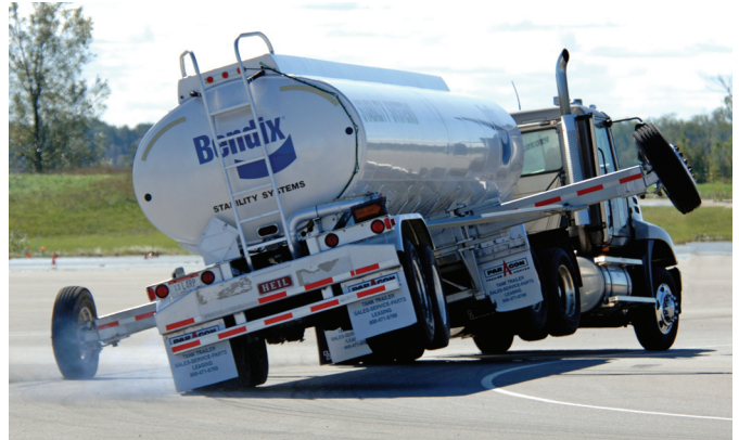
Does more than just rollover mitigation – Bendix ESP also addresses many of the "loss-of-control" situations that can lead to rollovers or other accidents.
