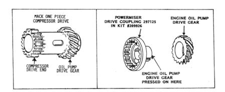
No. of Teeth on Oil Pump Gear of One Piece Drive
